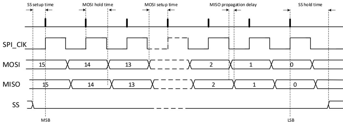
Figure 5.2. Timing diagram of SPI, CPOL=0 and CPHA=0.
