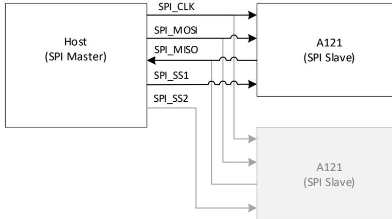
Figure 5.1. SPI master-slave connection.
