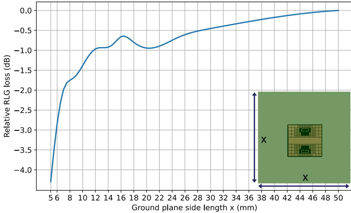
Figure 6.5. Simulated relative radar loop gain as function of ground plane side length ( $x$ ). Ground plane is a solid square ground plane.
