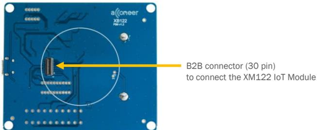
XM122 IoT module + XB122 Breakout board - Top view
