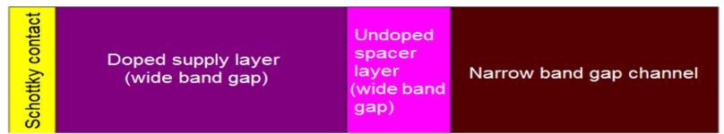
**Fig.2 Formation of 2DEG Quantum Well at AlGaAs/InGaAs heterojunction**
