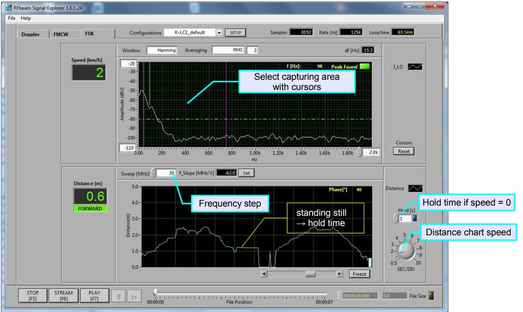
Fig. 20: FSK using K-LC1a: moving person, stopping for 1 second
