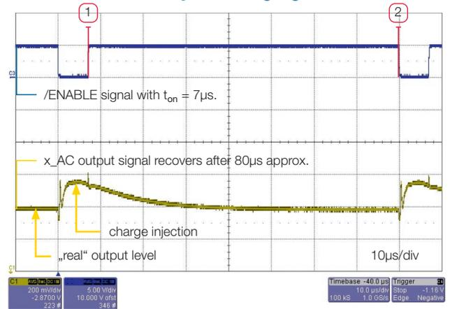
Figure 7: x\_AC output amplitude decreases during sleep time.
