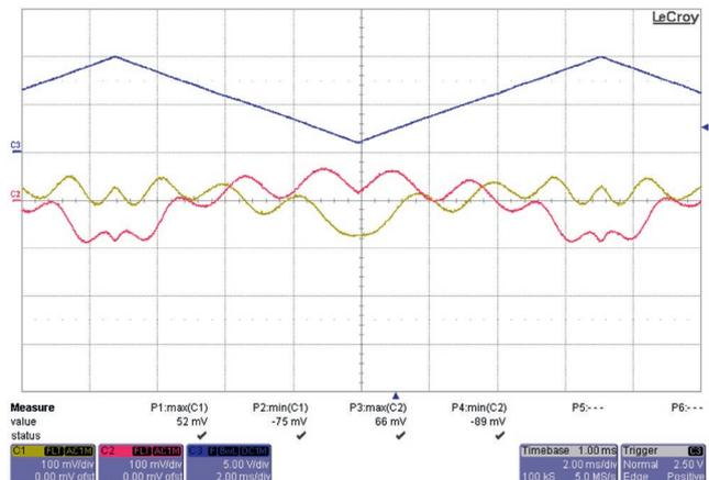
I\_AC and Q\_AC outputs show a low frequency caused by local carrier feedthrough.
